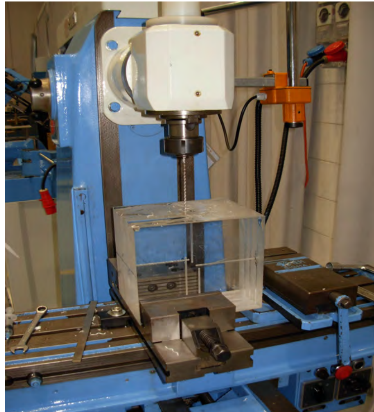
PMMA being drilled to get holes for thermocouples
