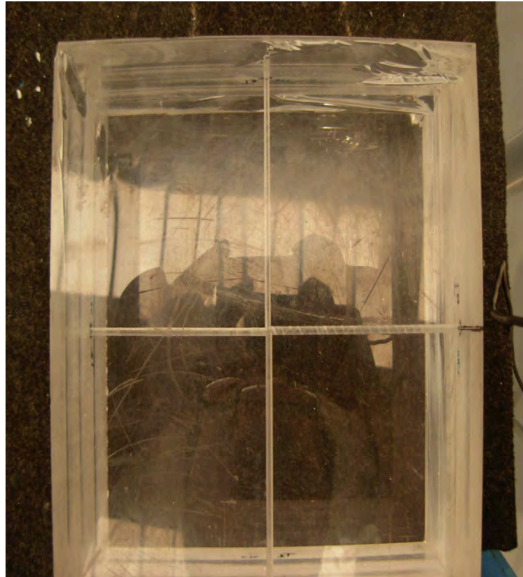
PMMA after drilling with holes for thermocouples
